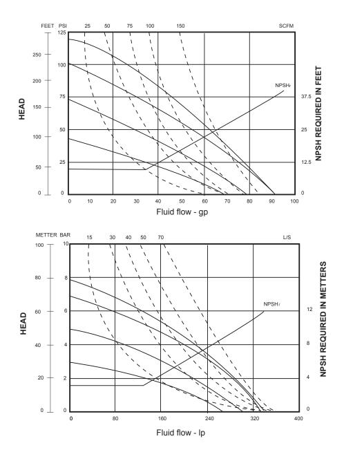
\*Performance is based on the following: elastomer fitted pump, flooded suction, water at ambient conditions. The use of other materials and varying hydraulic conditions may result in deviations in excess of 5%.
