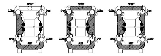
SKYLINK AODD pumps adopt compressed air for power source and depend on diaphragms which move left and right to reach the volume sealed working chamber to achieve loading and discharging.
